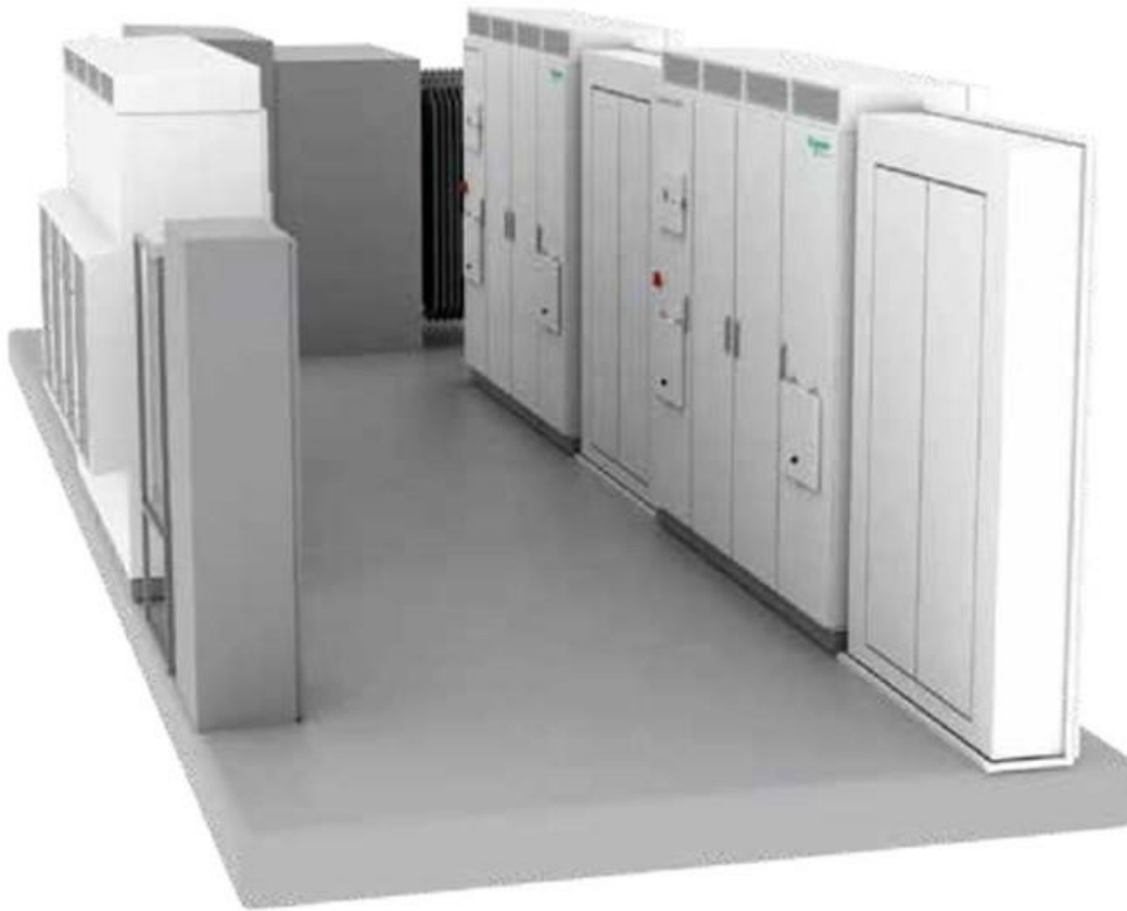
Figure 3-10 Example of a PV skid
